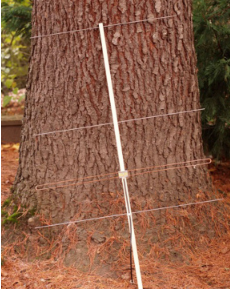
Square Yagi for 222.1 MHz 4 elements on 3/4" x 5/8" wood boom. 9.1 dBi gain, clean pattern
