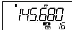
The display shows that memory channel 16 is set as a skip channel.
