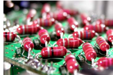
Large inductors in the RF stage
