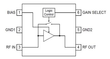
and the extra 3mm square MMIC would operate in the bypass mode on all bands except for 9 CM to provide a correct LO level for the Mixer. This was another aspect of the Rev C update. This MMIC is a LNA by design but has a P1dB of +27 dBm or so. With this performance, one can assume there may be other uses for this same component and will be discussed in the presentation of this paper.
