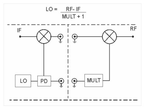
mixer through a filter/multiplier stage if required. The IF signal from the 5-24 GHz mixer will then be one that can be converted to the original 2 M signal derived from the same LO frequency in the multiband transverter. This will be discussed in the presentation but the math of it is simple to follow.
