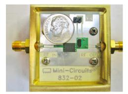
RF circuit board designers that now rely on machine assembled circuit boards can select economical linear 1+ Watt broadband MMIC's that will operate with a very flat gain response. A sample of one is shown to the left in an evaluation circuit. This Power Amplifier MMIC can be utilized in a multiband transverter covering all bands from 6M through 23 cm producing 1 watt of linear output with a flat gain not exceeding 15dB if the filtering is maintained. This component will be utilized in the
