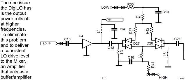
would be inserted between the two. This will then have an additional switchable attenuation circuit that would ensure the correct drive level per band of operation. This circuit is show above. When the LOW is biased, the PIN diodes switches in the "T" pad attenuator. When the HIGH is biased, no attenuation is in line.
