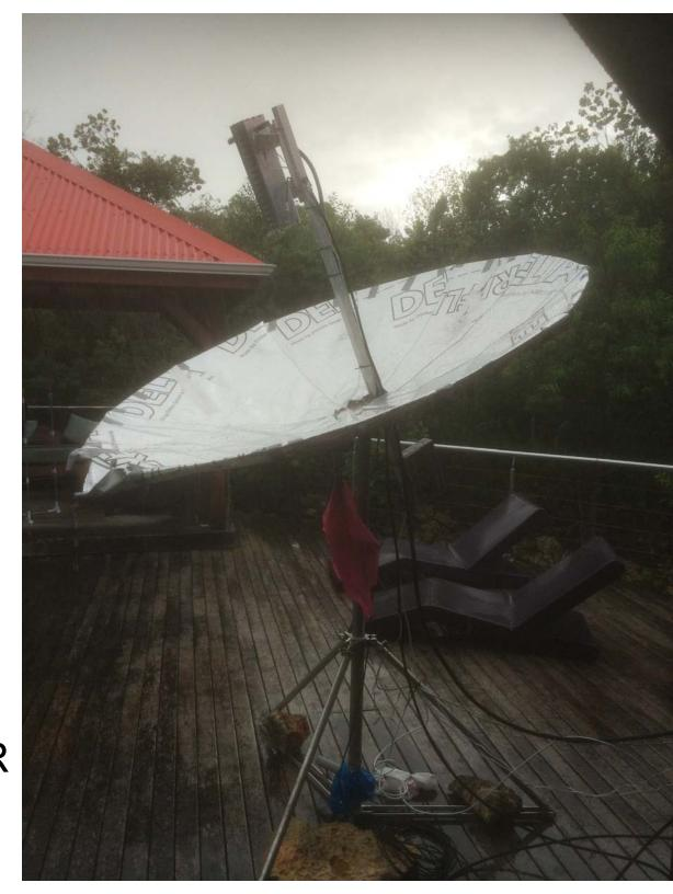
HERE IS THE DISH WITH THE 1296 FEED IN PLACE.
