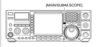
→ Push [MAIN/SUB•M.SCOPE] for 1 sec. to toggle the mini scope indication ON and OFF.
