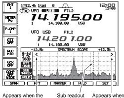
Appears when the Sub readout Appears when the marker is out of range. or TX marker marker is out of range.
