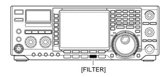
The filter selection is automatically memorized in each mode.
