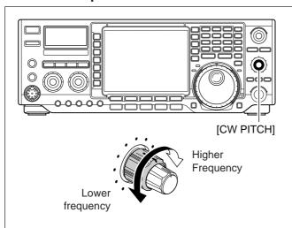
The received CW audio pitch and monitored CW audio can be adjusted to suit your preference (300 to 900 Hz in 25 Hz steps) without changing the operating frequency.
