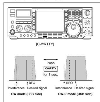
CW-R (CW Reverse) mode receives CW signals with a reverse side CW carrier point like that of LSB and USB modes.
