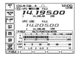
③ Push [METER] for 1 sec. or push [EXIT/SET] to turn the multi-function digital meter OFF.
