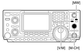
• [EXAMPLE]: Programming 7.088 MHz/LSB into memory channel 12.
