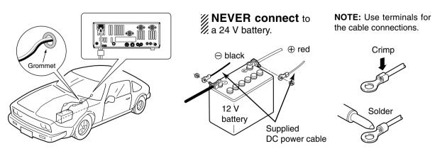
**NEVER connect** to a battery without supplied DC fuses, otherwise a fire hazard may occur.
