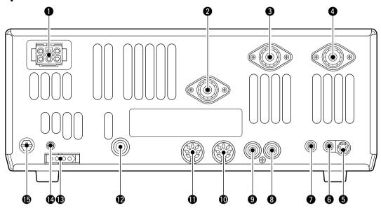
◆ DC POWER SOCKET [DC 13.8V] (pgs. 14, 16) Accepts 13.8 V DC through the supplied DC power cable (OPC-025D).
