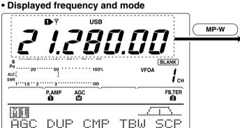
In this example, pushing [MP-W] enters 21.28000 MHz USB into the top memo pad and erases the oldest memo pad (21.34724 MHz LSB).
