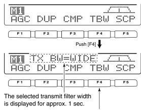
Push [F4] for 1 sec. to select the transmit filter width.
