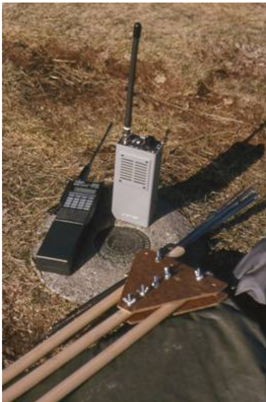
Figure 9 Mizuho 2m SSB/CW HT, Yagi Configuration
