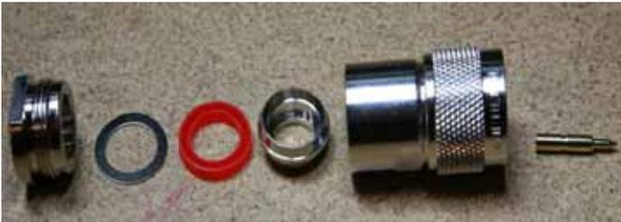
*Clamp-style N connector: The parts are shown in assembly sequence. The flat metal washer shown next to the nut is sometimes omitted (see text for details).*
