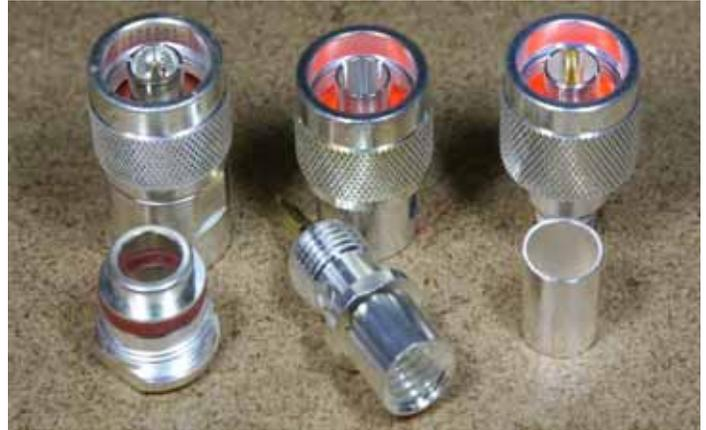
*The three common versions of the N connector (l to r): clamp-style, PL-259-style and crimp version.*
