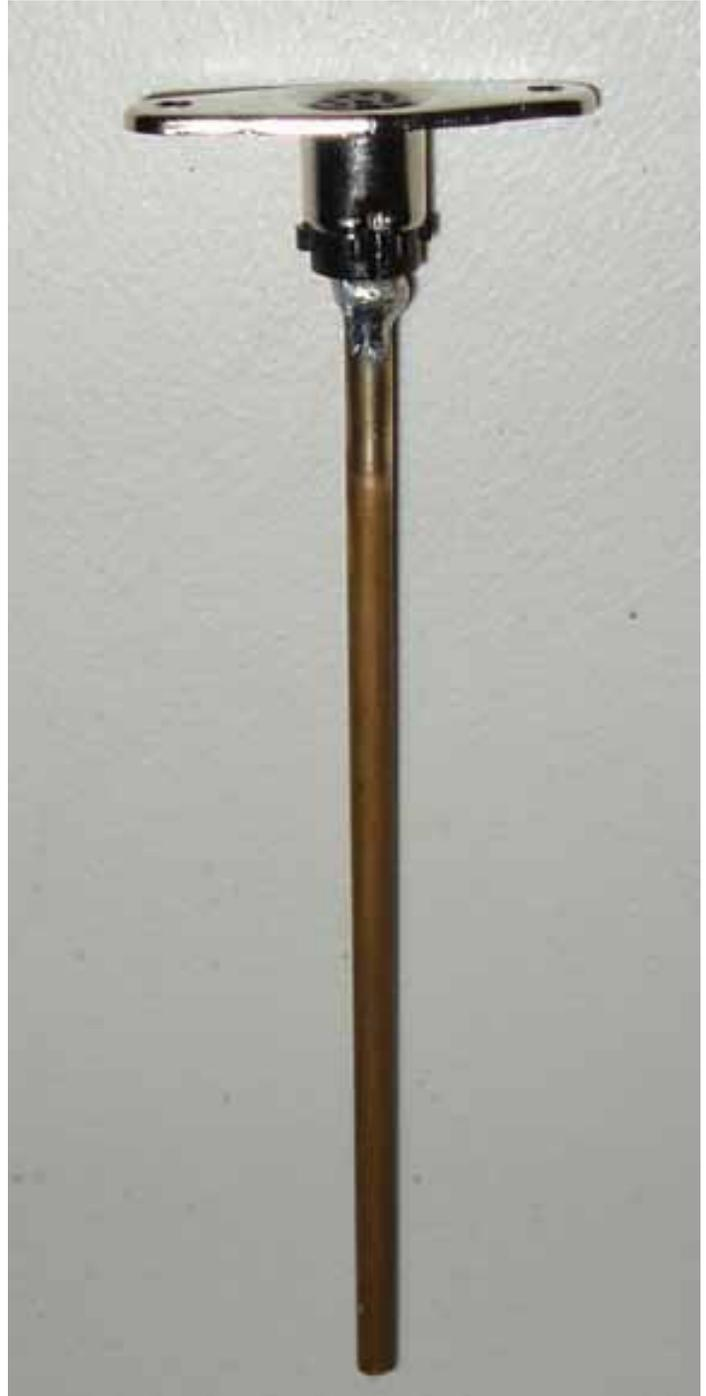
*N7CFO's DIN-connector soldering jig.*
