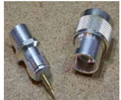
*PL-259-style N connector showing the parts separated.*
